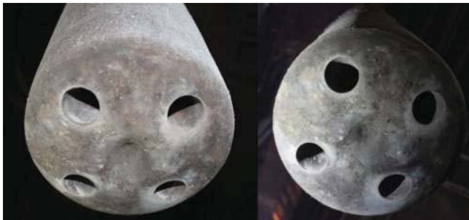
Figure 13 - Slagless Clean Up® after 611 heats around tip face.
