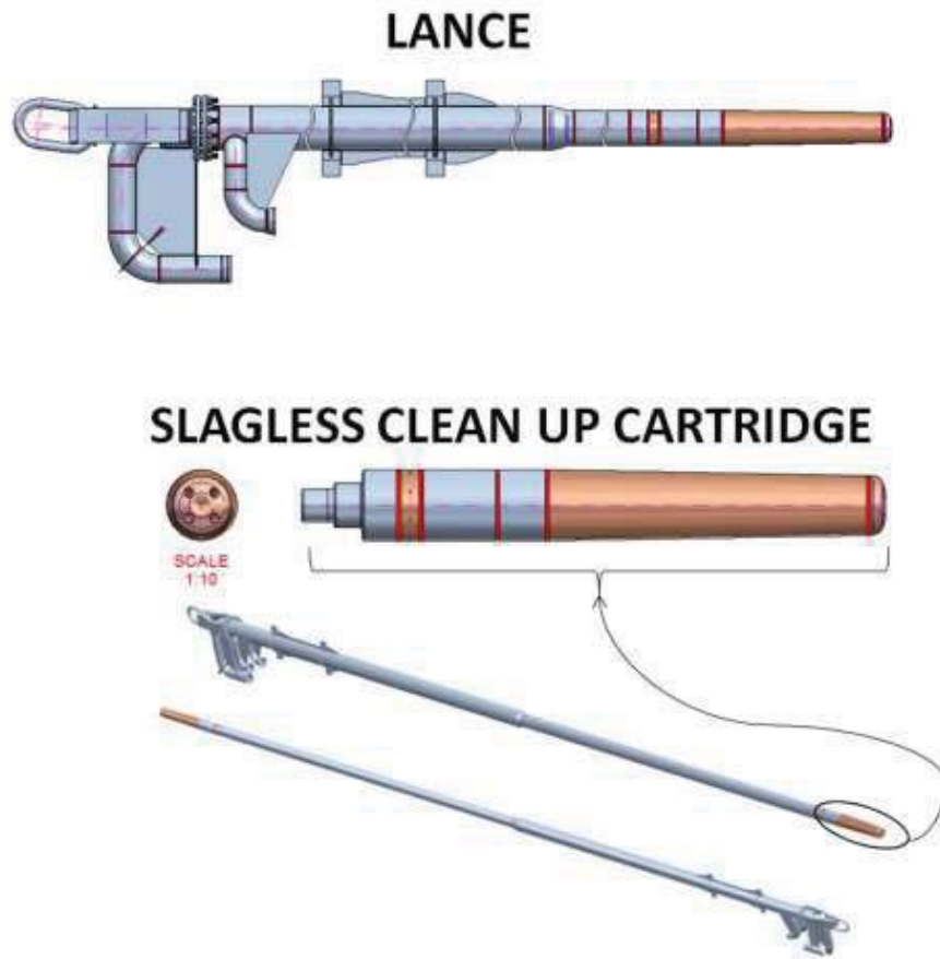
Figure 3 - Slagless Clean Up ® cartridge and assembly at top oxygen lance.
