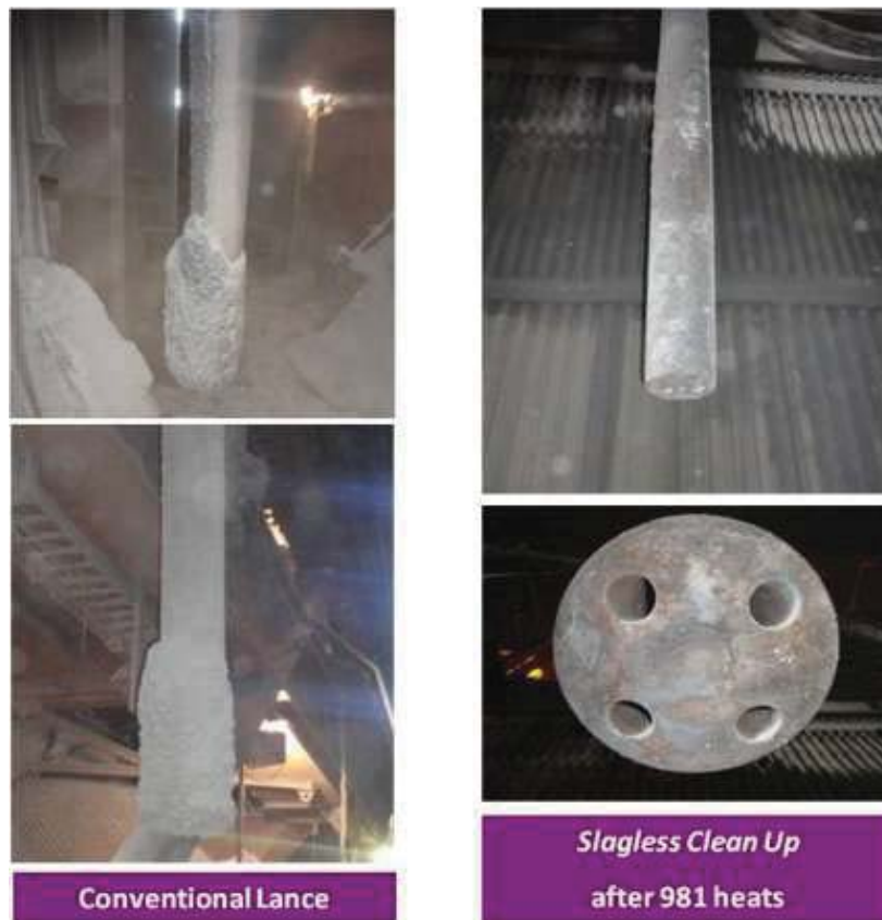
Figure 14 - Comparison between conventional lance and Slagless Clean Up ® after 981 heats. Conventional lance typical skull formation.
